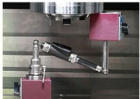
⑦、Ballbar roundness test, 300mm must be within 0.012mm to ensure the accuracy of the machine tool.
