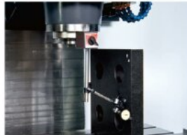
⑤、Perpendicularity parallelism test, test the parallelism and perpendicularity of each axis, within 0.01mm.
