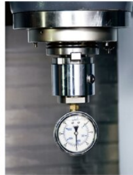
③、Spindle tension test to detect the broaching force of each spindle.
