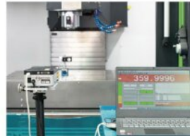
⑥、Laser detection, the accuracy of the full stroke movement has been corrected and compensated by laser to ensure the positioning accuracy and repeat positioning accuracy of the machine.
