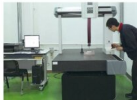
⑨、Each machine tool must be tested by the Hexagon CMM before leaving the factory.
