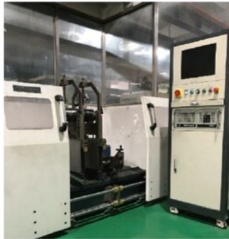
①、Spindle table type dynamic balance test to ensure spindle machining accuracy.
