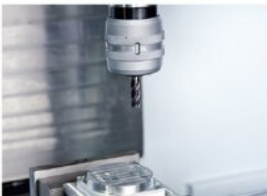
⑧、Processing inspection, each machine tool is made a standard test piece to inspect the processing accuracy.
