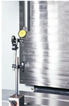
②、Spindle deflection test, 300mm is required to be within 0.005mm to ensure the accuracy and verticality of the spindle.
